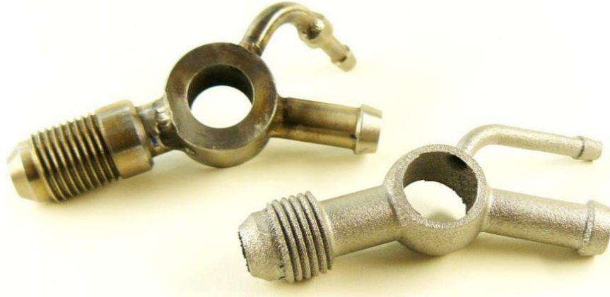
Figure 4: original welded part in comparison to LBM manufactured version 5
