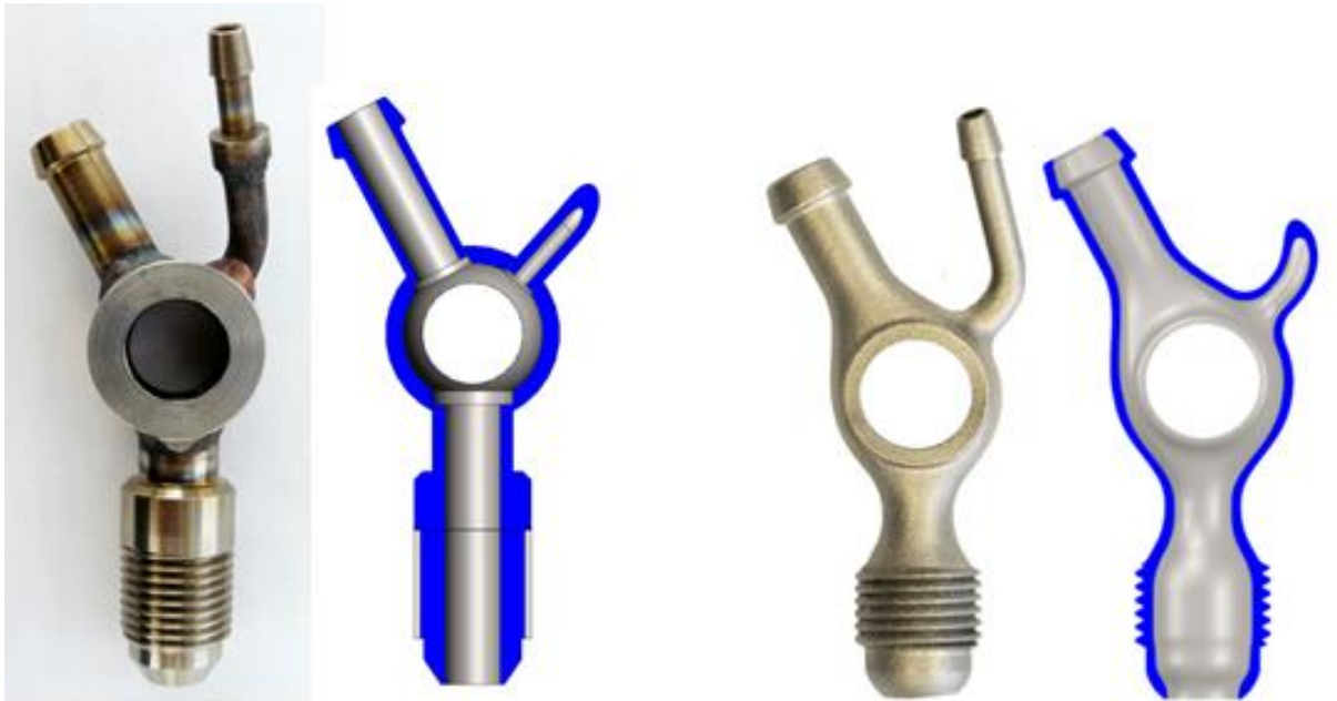
Figure 11: Full view and sectional view of original part and version 12 of the fuel collector
