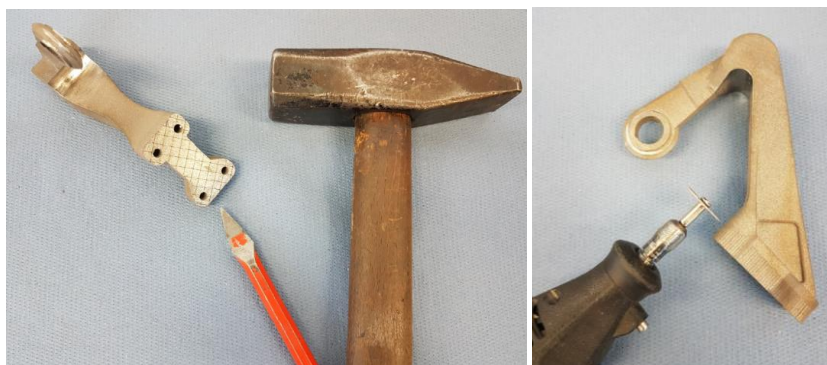
Figure 18: Manual Support removal with hammer and chisel (left) or dremel multitool (right) ©FOTEC
