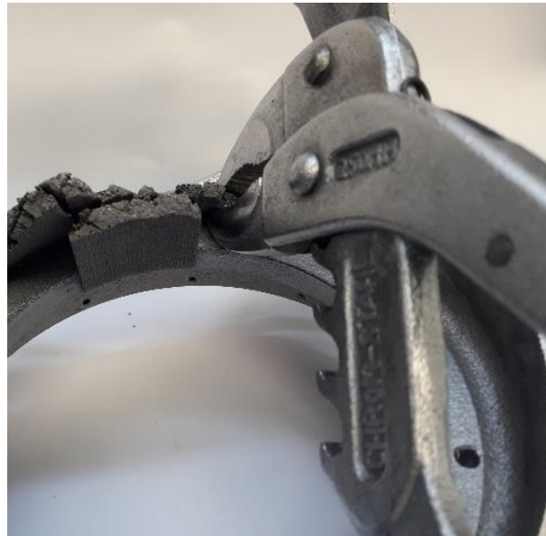
Figure 20: Breaking off support residues with water pump pliers ©FOTEC
