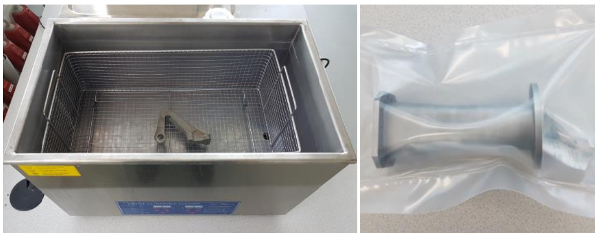
Figure 25: Cleaning in an ultrasonic bath (left) and packaging in vacuum-sealed bags (right) ©FOTEC
